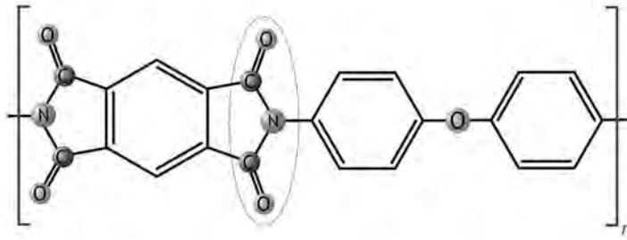
Figure 8.4 Kapton polyimide. The circled \text{NC}_2\text{O}_2 functional groups are the imide groups. The material contains oxygen (O), carbon (C), nitrogen (N) and benzene hexagons ( \text{C}_6\text{H}_6 ). The imide groups are prone to hydrolysis, and the material does not tolerate heat and moisture simultaneously
