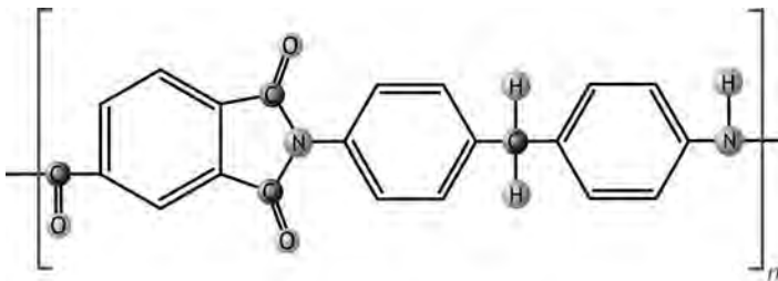
Figure 8.5 Polyamide–imide polymer. The material contains hydrogen (H), oxygen (O), carbon (C), nitrogen (N) and benzene hexagons ( \text{C}_6\text{H}_6 ). The imide groups are prone to hydrolysis
